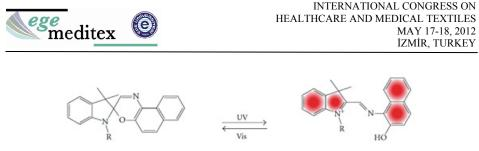
Figure 1. Schematic representation of photochromism mechanism [9]
