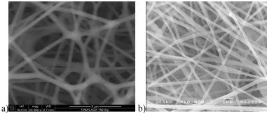
Figure 1. SEM microphotographs of electrospun nanofibers structures with addition of nano-sized hydroxyapatite: a) Sample 1 (magnification x 24000); b) Sample 2 (magnification x 10000)
