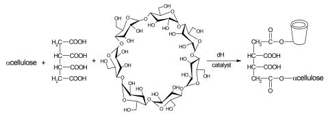
Figure 1. Schematic representation of the esterification reaction between cellulose and CDs via the polycarboxilic tetraacid, BTCA. The reaction occurs at high temperatures in the presence of catalyst.
