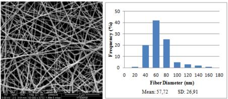
Figure 1.SEM images of PA 6 nanofibers and diameter distribution
