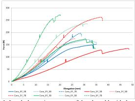
Figure 1. Load-elongation curves of developed braided structures
