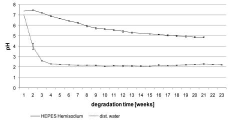
Figure 2. Changes in pH of the dissolution media during degradation of PGA at 37°C under static conditions
