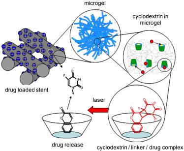
Figure 2. Project concept – RWTH Aachen University ERS Funded Project "Photorelease"
