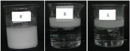
**Figure 1.** Photos of aqueous calcium carbonate solutions. (a) Uncoated calcium carbonate, (b) Coated calcium carbonate, (c) Coated breathable film grade calcium carbonate.
