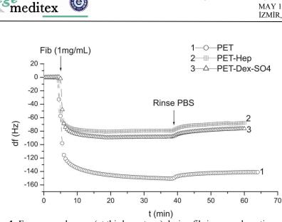
Figure 1. Frequency changes (at third overtone) during fibrinogen adsorption onto nonmodified (PET) and anticoagulant coated (Heparin, Dextran Sulphate) PET surfaces monitored by QCM-D (times of fibrinogen additions, as well as rinsing with buffer are market by arrows)
