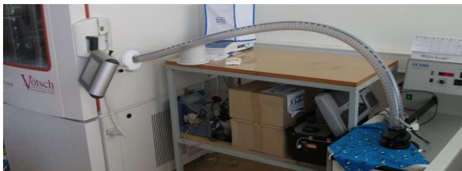
Figure 1. Measuring setup consisting of the source of hot and humid air VOETSCH, air permeability tester FX 3300 and the air temperature and humidity measuring system AHLBORN
